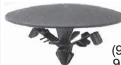
18746 (90700-SJ4-000) Black Nylon Hood Insulation Retainer Head Diameter: 30mm Stem Diameter: 15mm x 18mm Stem Length: 6mm Acura Legend 1991 - On Honda 1998 - On UNIT PACKAGE: 15
