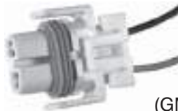
17109 (12085525, 12085527, 12085528, 12101895, 12117361) 3 Wire Alternator Harness Connector Two 18 gauge and one 12 gauge leads. Can be used to replace two wire and single wire harness connectors by taping (Do Not Cut) the appropriate unused leads. GM 1986-On UNIT PACKAGE: 1
