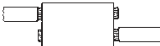
Parallel Connectors Proper Wire Insertion
